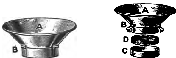
A —Body of Strainer. B —Clips to hold C and D in place. C —Compression Band. D —Wire Gauze.
